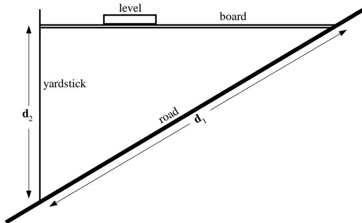
Mark out a longer  $\mathbf{d}_1$  on the road (about 30 ft), and calculate the new  $\mathbf{d}_2$  from  $\mathbf{G} = \mathbf{d}_2/\mathbf{d}_1$ . What work will you have to do to gain the elevation  $\mathbf{d}_2$ ?
