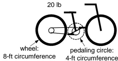
A bike weighs 20 lb, the circumference of its wheels is 8 ft, and the circumference of the pedaling circle is 4 ft. We define the gear ratio  $\mathbf{R}$  as the number of times  $N_w$  the wheels turn divided by the number of times  $N_p$  the pedals go around.
