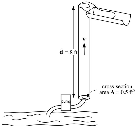
the pump must provide. The pump takes water from a stream and fills a pipe  $d = 8$  ft tall with a cross-section area of  $A = 0.5 \text{ ft}^2$  (the diameter is 9.5 inches). When the pipe is filled, it has  $(8 \text{ ft})\cdot(0.5 \text{ ft}^2) = 4 \text{ ft}^3$  of water. Since a cubic foot of water weighs 62 pounds, the total weight of the column of water is  $(4 \text{ ft}^3)\cdot(62 \text{ lb/ft}^3) = 248 \text{ lb}$ .
