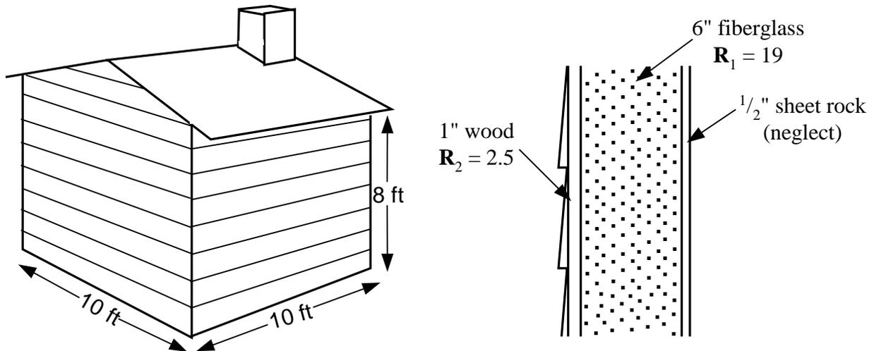
The thermal resistivity of fiberglass is  $R_1 = d_1 \times 3.2 \text{ (ft}^2\text{-}^\circ\text{F-hr/Btu)/inch}$ , where  $d_1$  is the thickness in inches. Since  $d_1 = 6$  inches,  $R_1 = (6 \text{ in}) \times 3.2 \text{ (ft}^2\text{-}^\circ\text{F-hr/Btu)/inch} = 19 \text{ ft}^2\text{-}^\circ\text{F-hr/Btu}$ .
